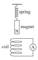
The magnet is pulled down until its north pole is just at the top end of the coil. The magnet is released and initially accelerates upwards away from the coil.
