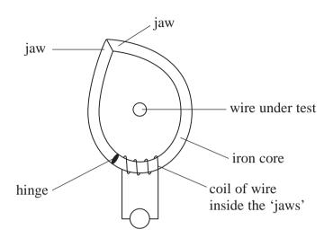
The 'jaws' of the clamp are opened, placed around the wire carrying the current and then closed. Inside the 'jaws' is an iron core with a coil of wire wrapped around it.
